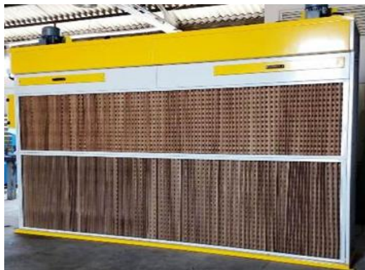
• DRY FILTERED PAINT EXTRACTION WALLS
